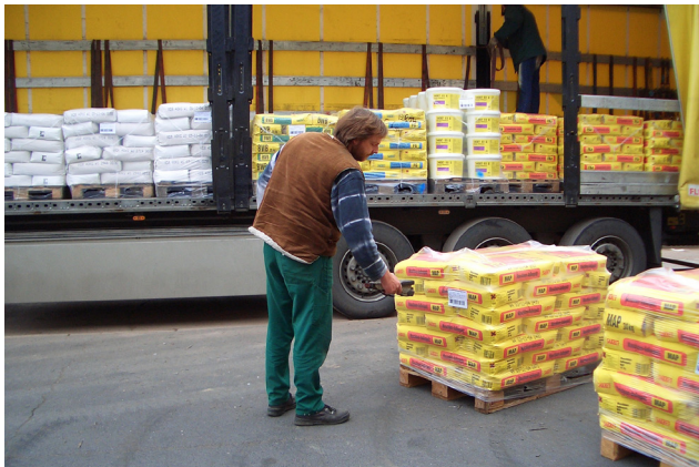
Staff in the dispatch zones of SAKRET's three German manufacturing plants are equipped with handheld radio data transmission terminals that scan barcodes and are constantly online.
