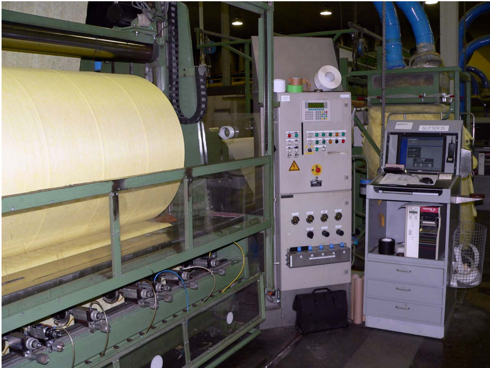
The workstation with scanner, screen and label printer next to a slitter machine in PGI's manufacturing department.
