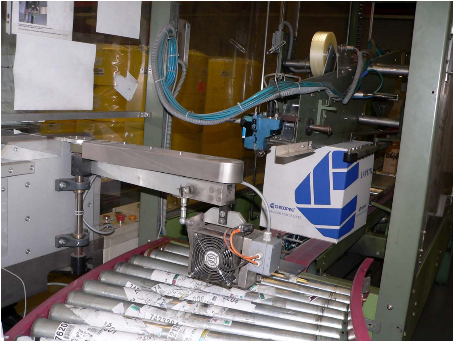
The Padlocker auto case sealer closes the product boxes with tape.
